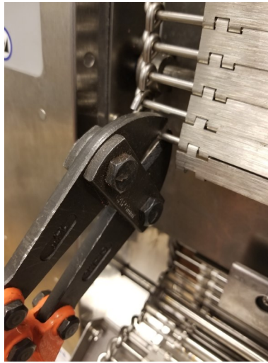
Cut the bottom wire using the bolt cutters.
