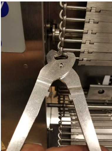
Open the hooks on the bottom link on both sides using the belt tool.
