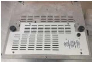
**3** Remove the 4 screws used to secure the control panel components via the Philips screwdriver, and turn over the control panel components.
