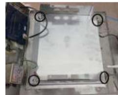
**7** Install the new heating plate into the equipment and assemble the dismantled parts in reverse steps.
