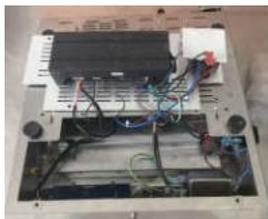
**4** Unscrew the retaining nut using a socket wrench. Turn over the main circuit board and unplug the connecting wire connector of the circuit board.
