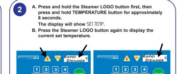
The CAL TEMP mode is used to calibrate the platen temperature with an external meter connected to the meter plug inlet on the bottom right side of the unit. Add ± 5°C (± 10°F).
