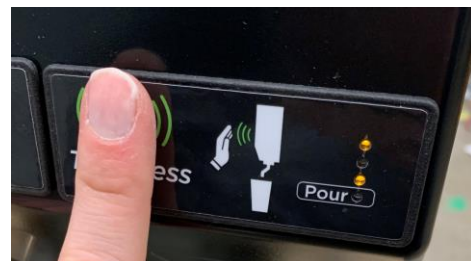
Finger shown to block sensor window and go into cleaning mode.
