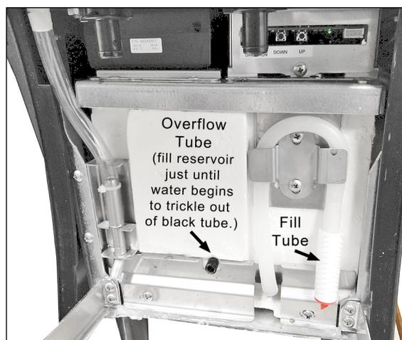
Figure 4-2 - Ice Bank Fill & Overflow Tubes
