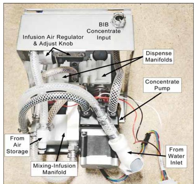
Figure 3-14 - Mixing-Dispensing Assembly
