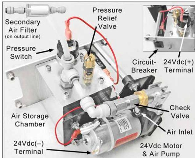
Figure 3-10 - Air Compressor and Air Storage
