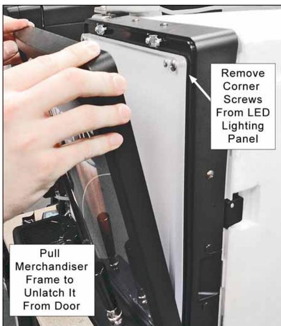
Figure 6-10 - Merchandiser LED Backlight Removal
