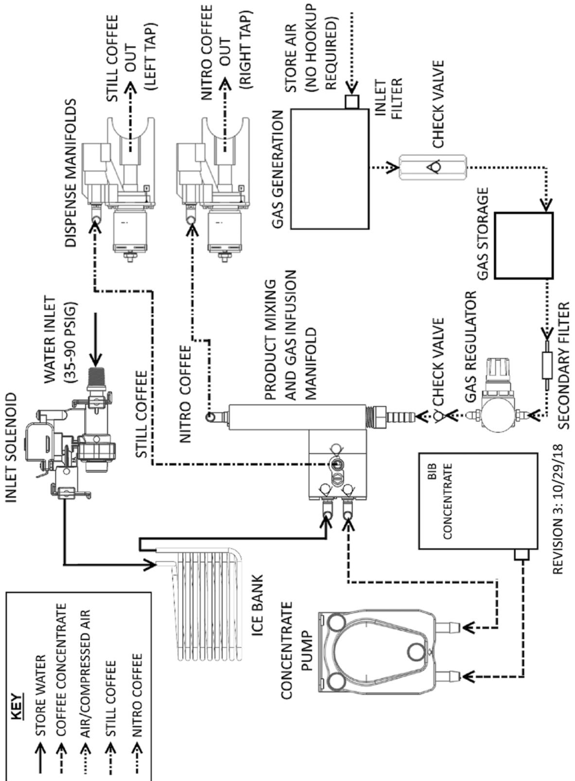
Figure A-1 - Plumbing Diagram
