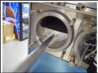
The bottom of the tool with the ramp going up should always go into the barrel first.
