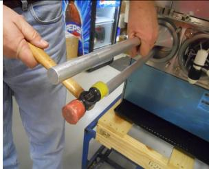
Then tap the bottom of the tool alternating between the top and bottom tool. Continue until tool travels through the entire barrel. Check the barrel to see if the bump is removed. Repeat steps (4-6) until all the bumps have been removed.
