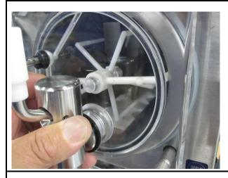
Install Face Plates. Verify Spinner does not block Blades. Insert spinner at 3 o'clock and 9 o'clock to prevent interference.
