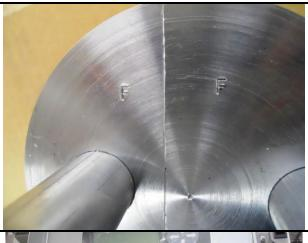
NOTE: Bump Fixtures must be kept together as sets to work properly each set or pair has a letter on top to show its corresponding side.
