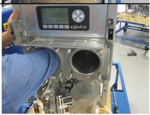
With a clean towel, dry the inside of the barrels completely. Use a flashlight to inspect the barrel and make sure there is no product or moisture remaining. Check the barrel for bumps to prepare for repair.
